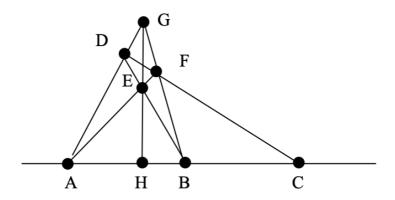
**Example 3:** There's a straight road which ends at the base of Uluru (Ayers Rock) in Central Australia. It is desired to continue the road on the other side of the rock so that both portions are in the same straight line. How can this be done using only standard surveying equipment which can effectively draw a straight line between two points (provided the rock is not in the way)?
